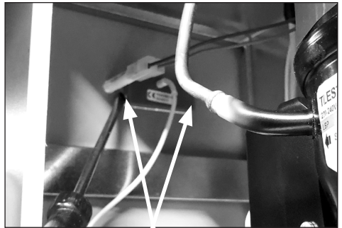
5. Use a screw driver to gently push the socket of the thermometer.
