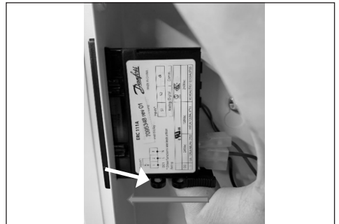
11: Use your finger to press and slide the upper clamp back in place to secure fixture of the thermostat
