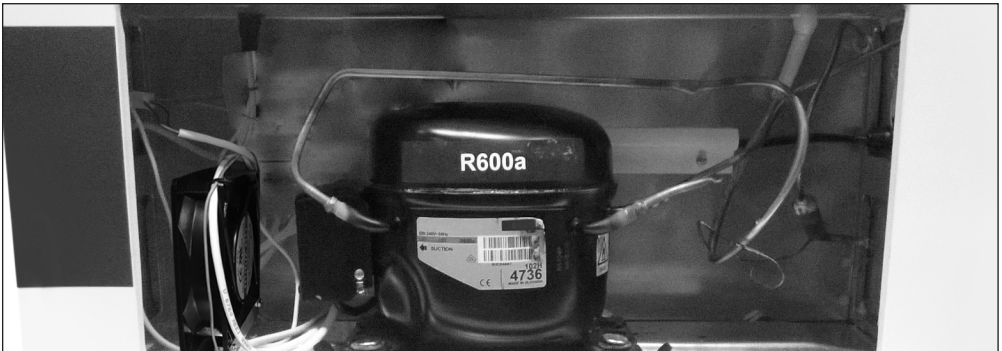
The starting device is mounted on the left side of the compressor.
