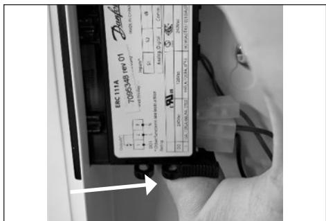
5: Use your finger to press and slide the lower clamp backwards to remove from the thermostat body
