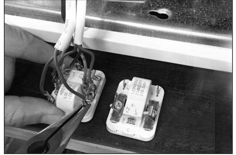
8. Use a nose plier to unmount the wire sockets from starting device.
