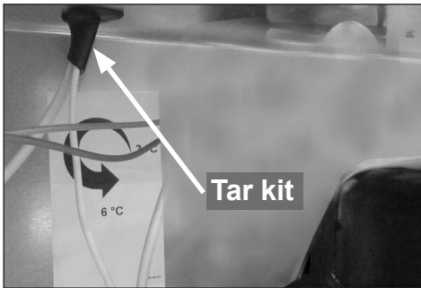
12. IMPORTANT! When re-mounting the new thermometer remember to properly seal the wire feed through.
