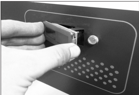
8. Installation of thermometer display.
