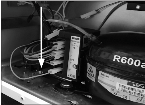
2. Loosen the 2 screws with a torx 20.
