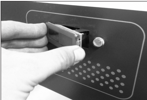
8. Installation of thermometer display.
