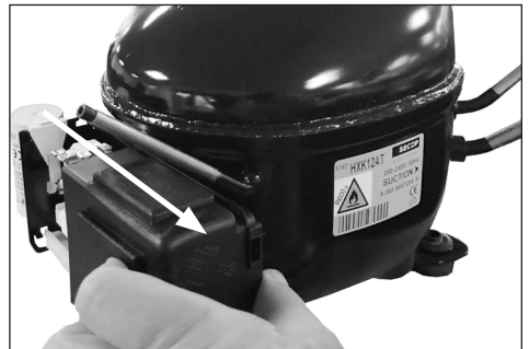
The starting device is mounted on the left side of the compressor.
