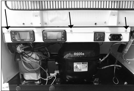
1. Access electrical components Dismount 3 x Torx 20 screws and unmount the junction box lid
