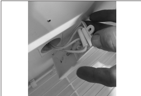
12. IMPORTANT! When re-mounting the new thermometer make sure the wire sealing plug is placed properly.
