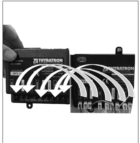
4. Exchange the wires from the old ECU to the new.
