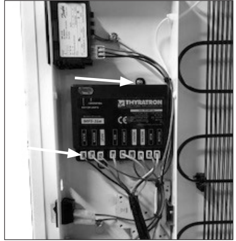
2.Loosen the 2 screws and remove the wires
