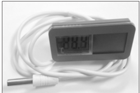
7. Thermometer comes with display, wire and sensor
