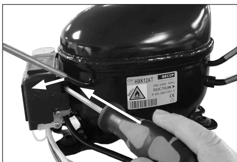
1. Dismount the cover by pushing the cover lock from right to the left with a flat screw driver.
