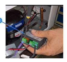
7: Exchange the wires 1/1 from the old thermostat to the new
