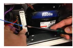
3: Unclick plactic cover/starting device from compressor bracket
