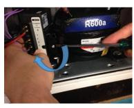
4: Use a screwdriver to disconnect the socket from compressor
