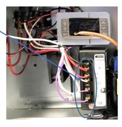
3: Gently pull out the thermostat bracket, by tilting out from bottom
