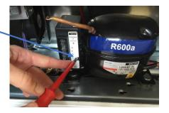
2: Place a screwdriver in the small vent in the plastic cover
