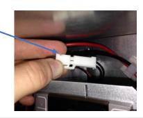
5: Remove black sealing tar-kit and gently pull the black wire until the probe is visible
