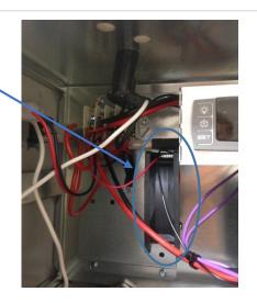
2: Unplug the power and signal wires form the ECU using a nose plier
