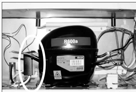
The starting device is mounted on the left side of the compressor.
