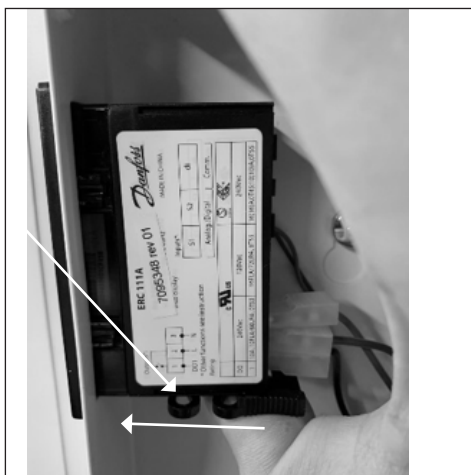
10. Put the thermostat back in place
