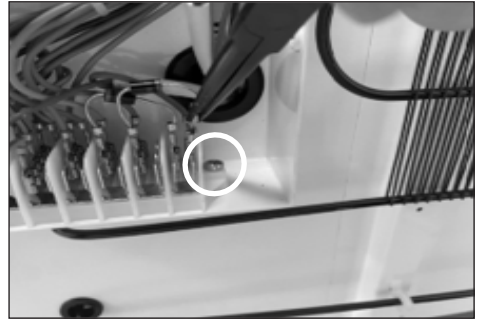
5. Remount the new diode with a nose plier by pushing the 2 x spade connectors on to the spades on the connection board
