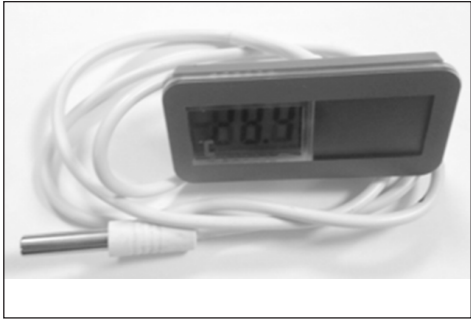
9. Thermometer comes with wire, PV solar cell, display and sensor
