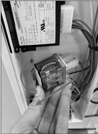
4. Turn the relay out from the left fixing bracket. Then slide it out from the right fixing bracket.
