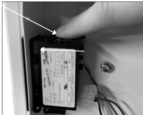
11. Use your finger to press and slide the upper clamp back in place to secure fixture of the thermostat
