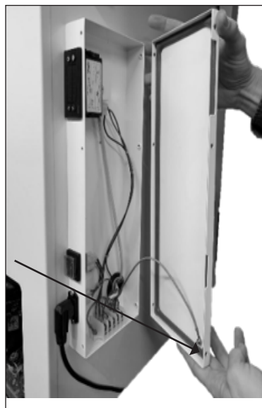
2. Remove grounding cable from junction box by unscrewing bolt with a wrench 6mm.
