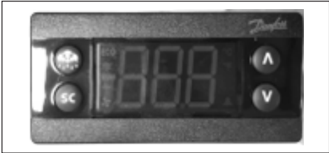
Danfoss controller: Front with display and adjustments buttons
