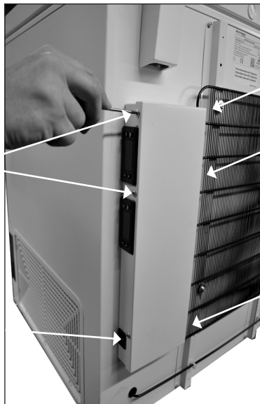
1. Access to electrical components Dismount 6 x Torx 20 screws and unmount the junction box lid
