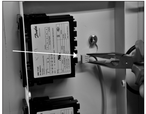
6. Pull out sensor wire from the socket
