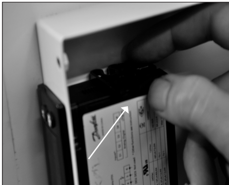
8. Slide the fixing clamps backwards
