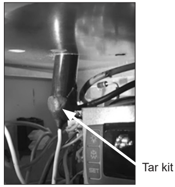
7. IMPORTANT! When re-mounting the new thermometer remember to properly seal the wire feed-through
